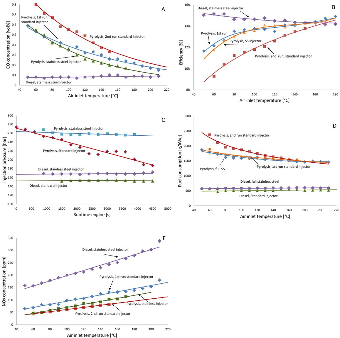
Figure 6<sup>A-E</sup>: Performance of the diesel engine at a load of 3 kWe as a function of the air inlet temperature for diesel and pyrolysis oil using a standard injector and a new stainless steel injector. In figure 6C the injector pressure is given as a function of the runtime of the engine
