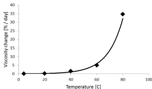
Figure 3: Relative change in kinematic viscosity [%/day] as a function of the storage temperature (pine derived pyrolysis oil).
