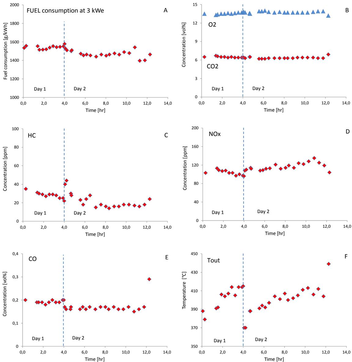
Figure 8<sup>A-F</sup>: Engine performance as a function of the time on stream for pyrolysis oil fuelling. Engine load = 3 kW<sub>e</sub>. Air inlet temperature = 150 °C.
