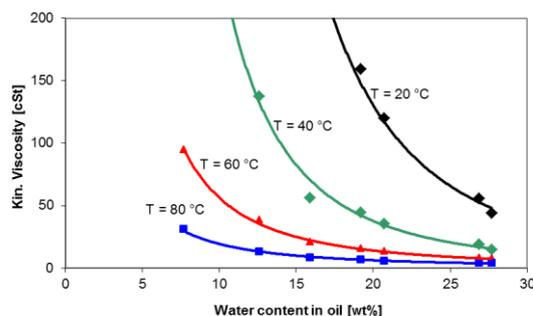
Figure 2: Kinematic viscosity of pyrolysis oil as a function of the water content in the oil and for different temperatures.
