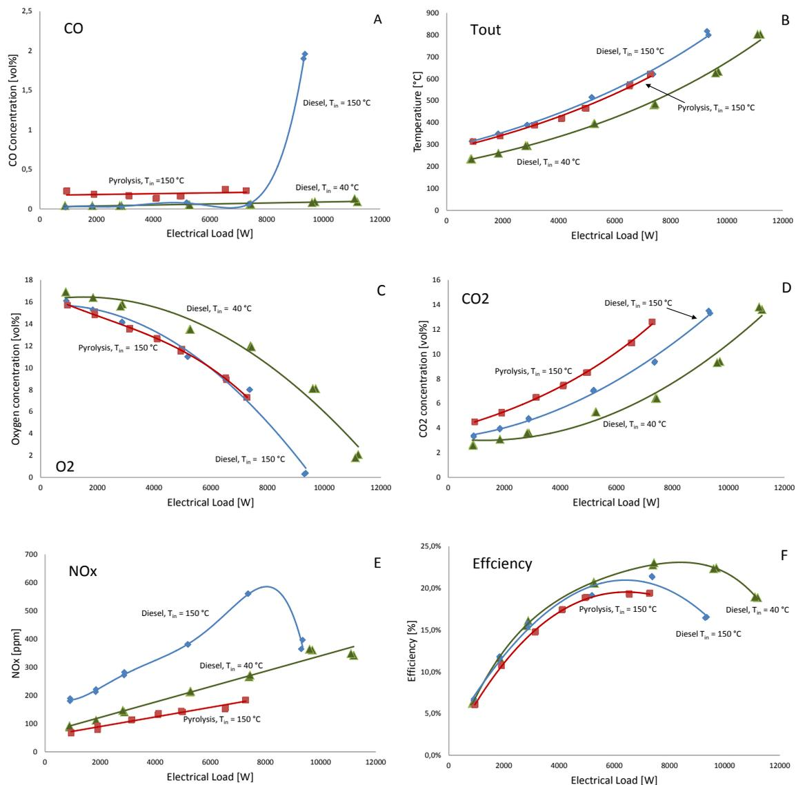
Figure 7<sup>A-F</sup>: Engine performance and flue gas emissions as a function of the electrical load for diesel and pyrolysis oil at different air inlet temperatures.
