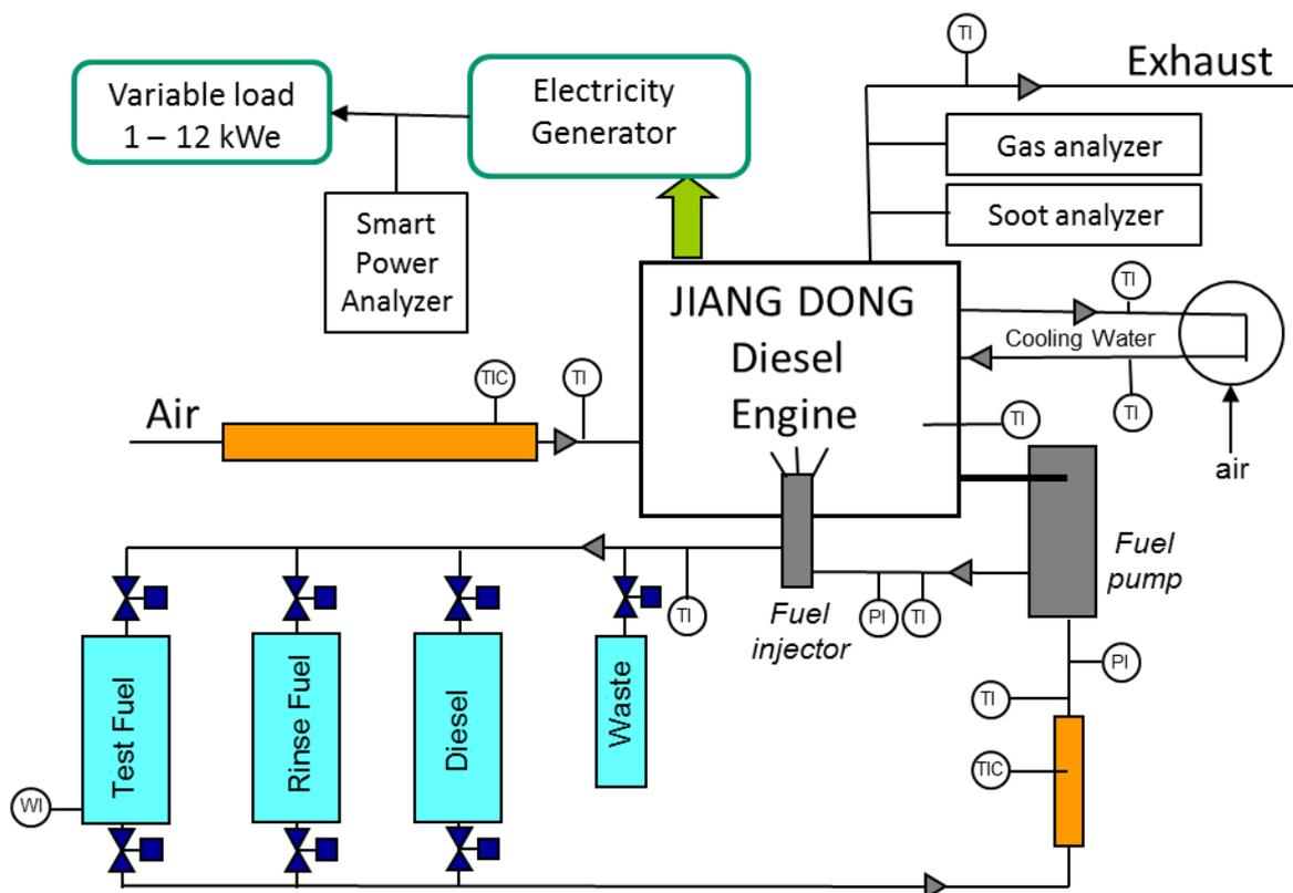
Figure 4: Schematic drawing of the engine test set-up
