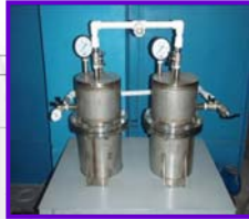
Sorption module clean energy oils
