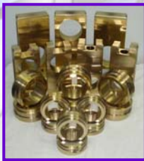
Experimental batch of items, shut-off and control valves, coated
