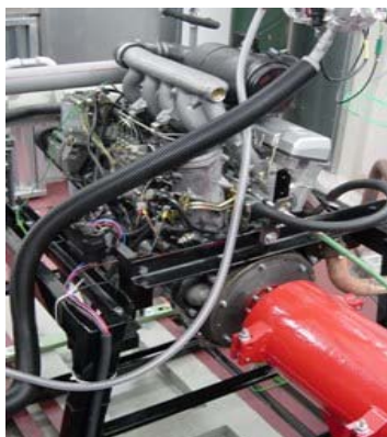
IDI VWP Test engine at Test bench Technical University Munich (TUM)
